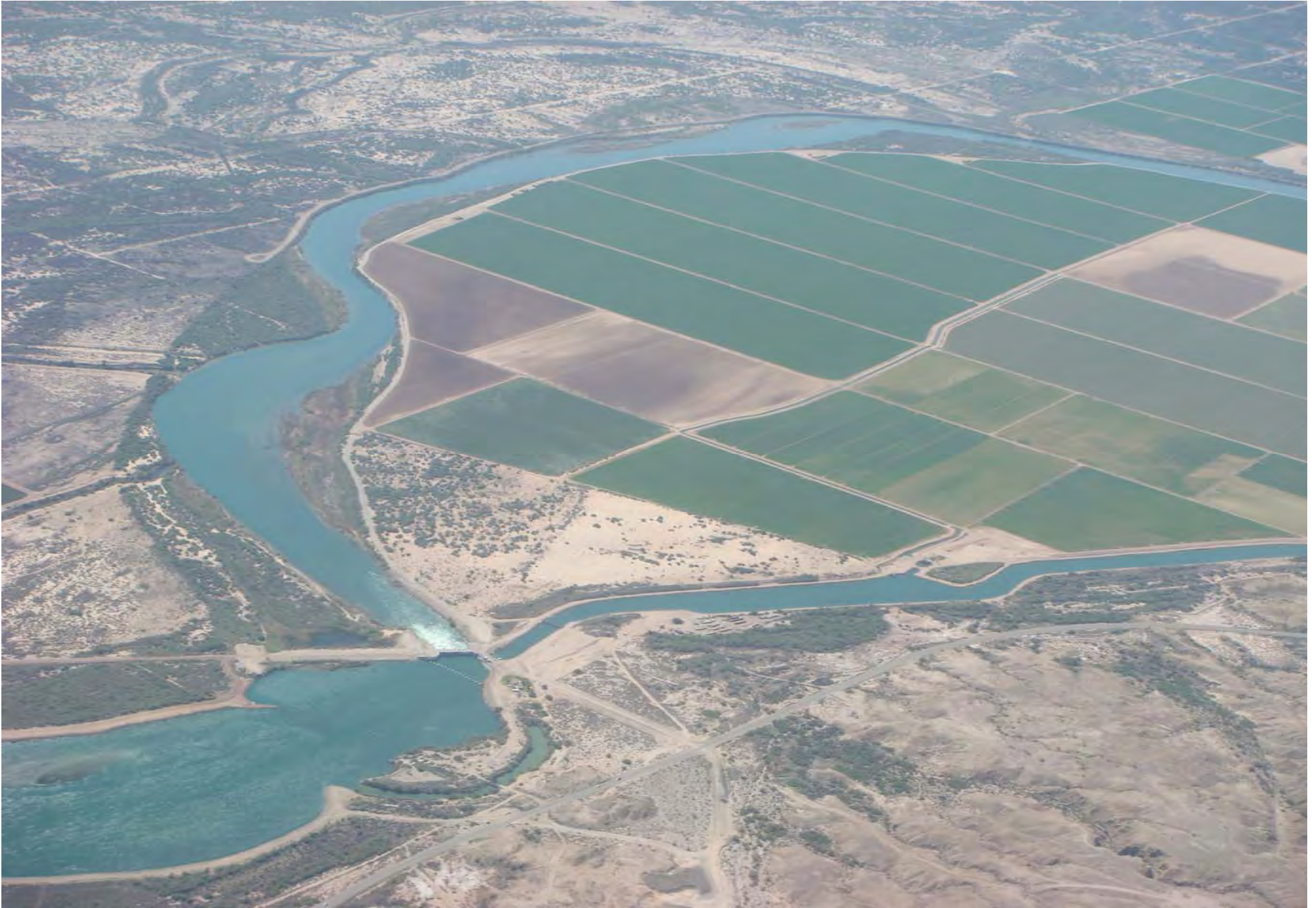
Palo Verde Diversion Dam diverts water from the Colorado River to the Palo Verde Irrigation District to supply water for 121,000 acres of valley and mesa lands.
